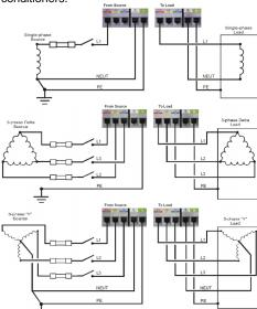
Just insert the IPC between your AC source and your AC load. The IPC is happy with any nominal voltage between 100V and 480V, and currents up to 200 amps per phase (continuous). Both 50 Hz and 60 Hz will be accepted by any IPC. And the IPC generates true phase-to-phase sags, not simulated phase-to-phase sags generated by some other sag generators.
