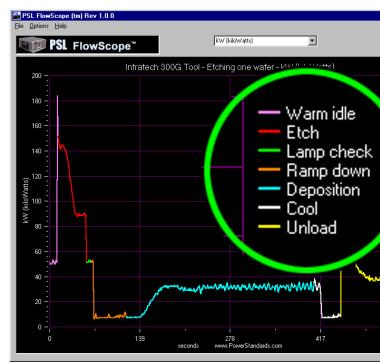
The Power Flow Analysis option turns the IPC into a powerful power flow recorder, meter, oscilloscope, spectrum analyzer, and vector scope. Record kW, kVA, kVAR, PF, THD, phase angles, and more, all optimized for analyzing power consumption in industrial equipment. Easily added to any IPC.
