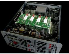
The IPC uses advanced, patent-pending switching technology to generate perfect voltage transitions. Special new technology permits 480V, 200 amp, 3phase control in a single, clean, portable package less than 9 inches (23 cm) high.
